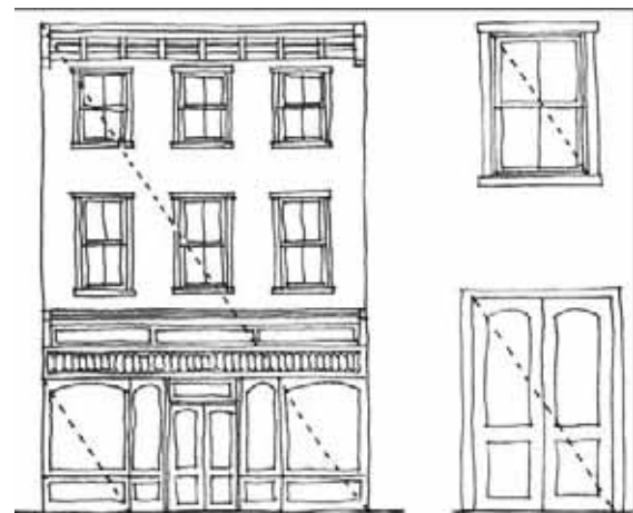
Analysis of a three-story commercial building façade showing the repeated proportions in façade elements, beginning with the overall façade and carried down to the proportions of individual glass panes. (Geometrically, when the diagonals of rectangles are parallel, the rectangles are proportional.)
