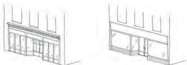
Two storefront designs for the same building. The left design is not a literal reproduction of a period storefront, but its scale relates to historical storefronts. The right storefront lacks human scale and vertical proportions.
