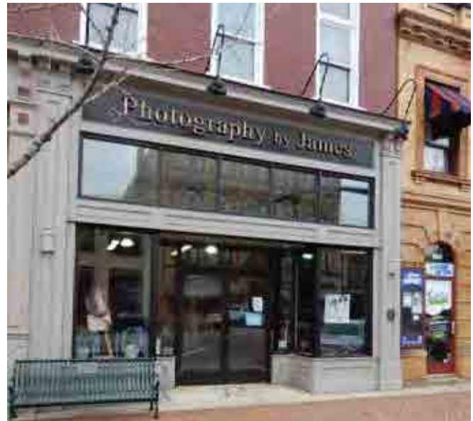
Projecting gooseneck lights fixtures illuminate the store-fronts without glare. The period form of the fixtures contributes to the character of the retail establishment during the daytime as well as after dark.
