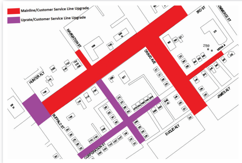
The map shows an overview of the Columbia Gas infrastructure upgrade in Beaver Borough. The red indicates the streets and area where the Company will fully replace the mainline and customer service line. The purple indicates where minimal construction will take place to upgrade existing facilities.
